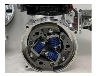
Always adjust the 3x nuts evenly and check the spring lengths after clutch adjustment to make sure they are all the same length (with proper Vernier calipers)
