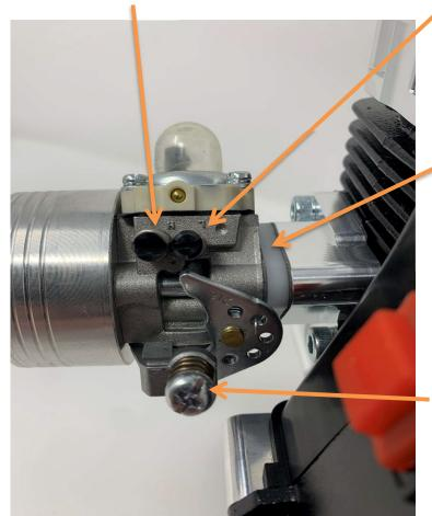
Heat isolator with high temp gasket fitted either side (supplied)
